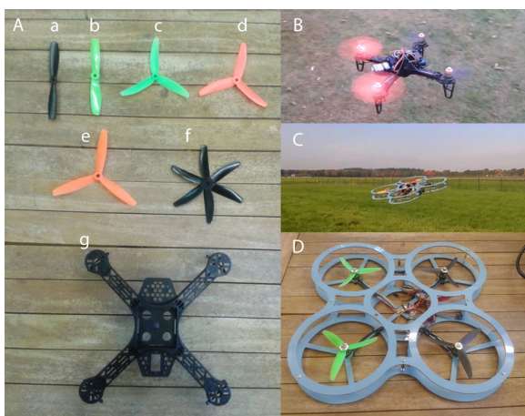
Figure 16: First simple prototype used for gaining insight and performing measurements. In A, the different tested propeller configurations are shown. In B the assembled original frame, performing a flighttest, is shown. In C and D our first produced prototype is shown.
