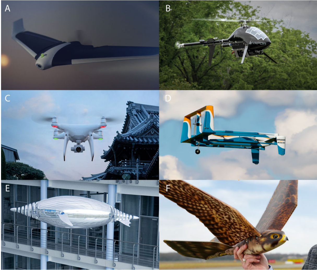
Figure 2: A selection of UAV types. A: Parrot Disco FPV, B: Pulse Aerospace HeliSynth, C: DJI Phantom 4 Pro, D: Amazon Prime Air, E: Festo AirPenguin, F: Clear Flight Solutions Robird
