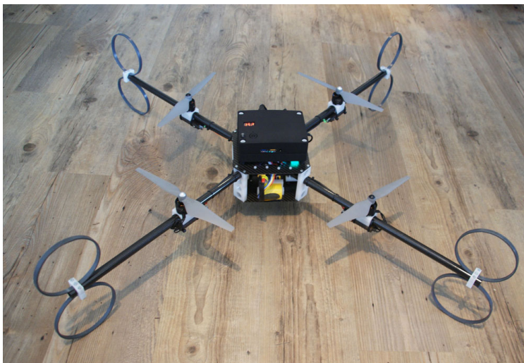
Figure 29: Overview of the produced finished product. The frame consist of CFRP tubes and plates. The frame components are connected by (white) HDPE blocks containing all the difficult form transitions and are easy to produce using milling techniques.
