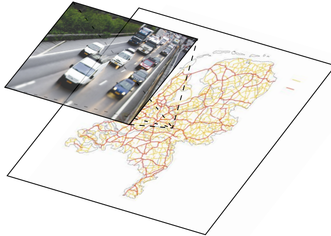
Figure 2.10: The motion problem of driving a car from A to B that can be abstracted to global planning on a map and local planning on the highway.
