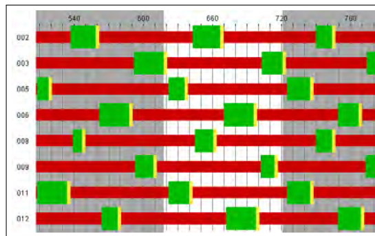
Figure 7.4: Phase diagram of a non-flexible order: no signal from the next block can start before the entire previous block has ended.
