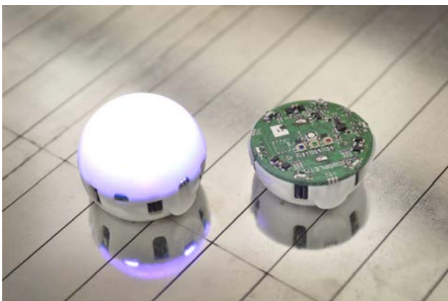
Figure 2 Swarm robots at the University of Colorado called the “droplet”, each about 2.5 cm in diameter. One to the right has the cover off, showing the internal features such as the electronics circuit board
